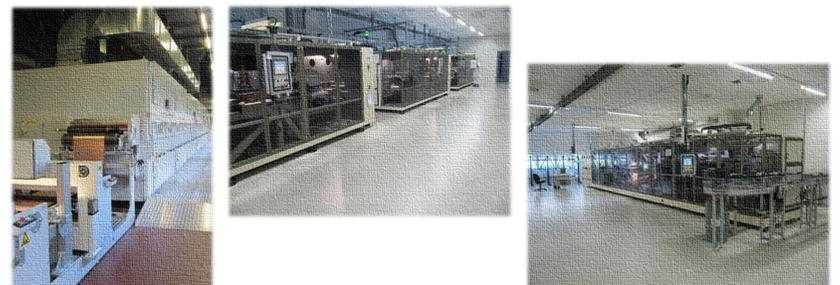
Fabrication steps: a part of coating line, electrode notching and cell assembly machines
