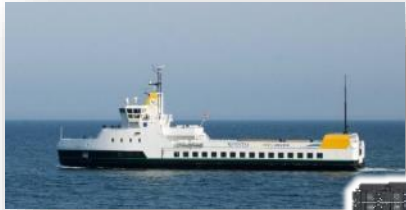
Ellen e-Ferry Ro-Pax vessel System energy: 4.3 MWh
